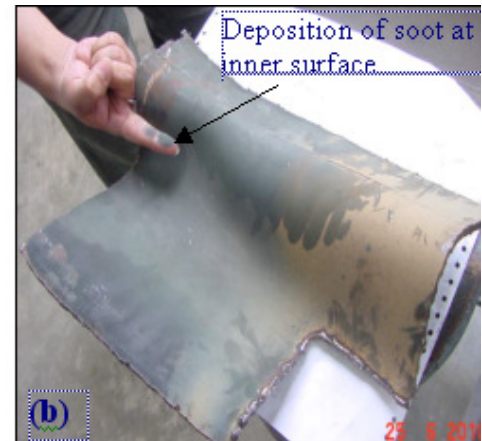
Fig.2 (a) Sample collected from bulged out part, (b) Deposition of soot at the inner surface
