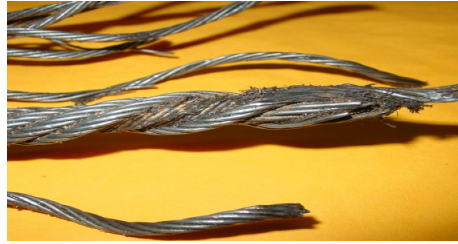
Fig.4 (b) ROPE SHOWING DECOLOURISING DUE TO FRICTION HEATING
